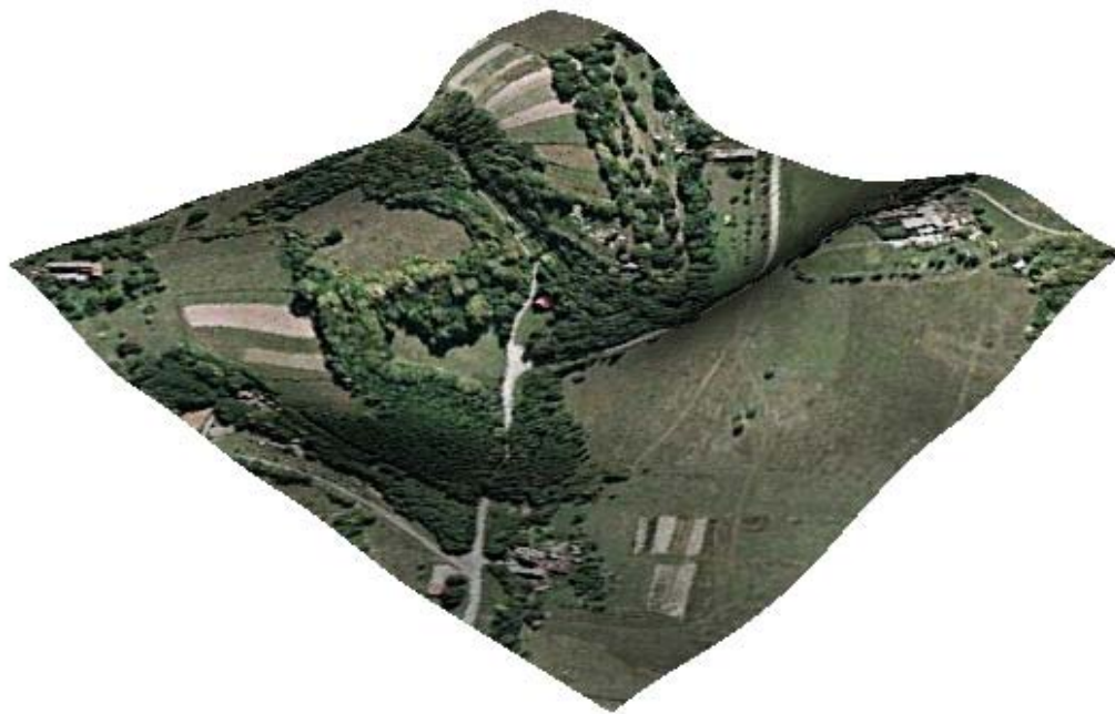
Picture 4. A satellite photo mapped as a texture onto the NURBS surface
