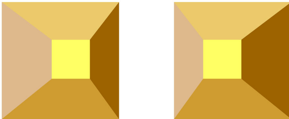
Figure 6. A pair of stereo images can be made by reflection and recolor of a graphical object
